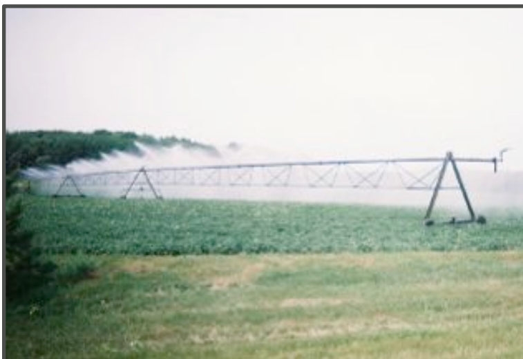
Figure 3: Application of pesticides to potatoes is frequently conducted by chemigation using center-pivot irrigation rigs.
